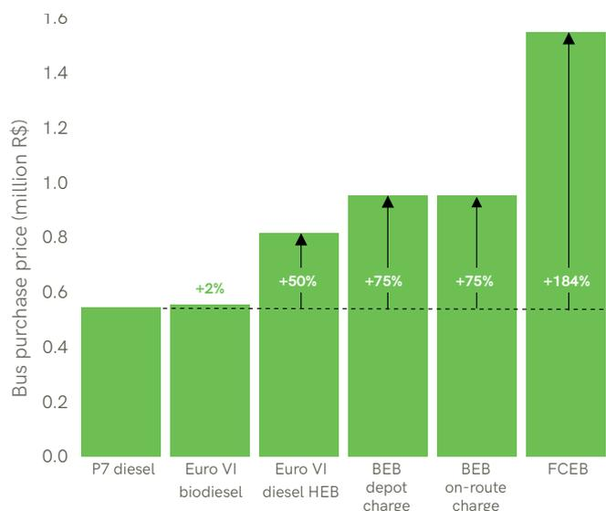
Figure 5-1 | Purchase price for electric drive transit buses compared to a conventional diesel bus<sup>40</sup>
